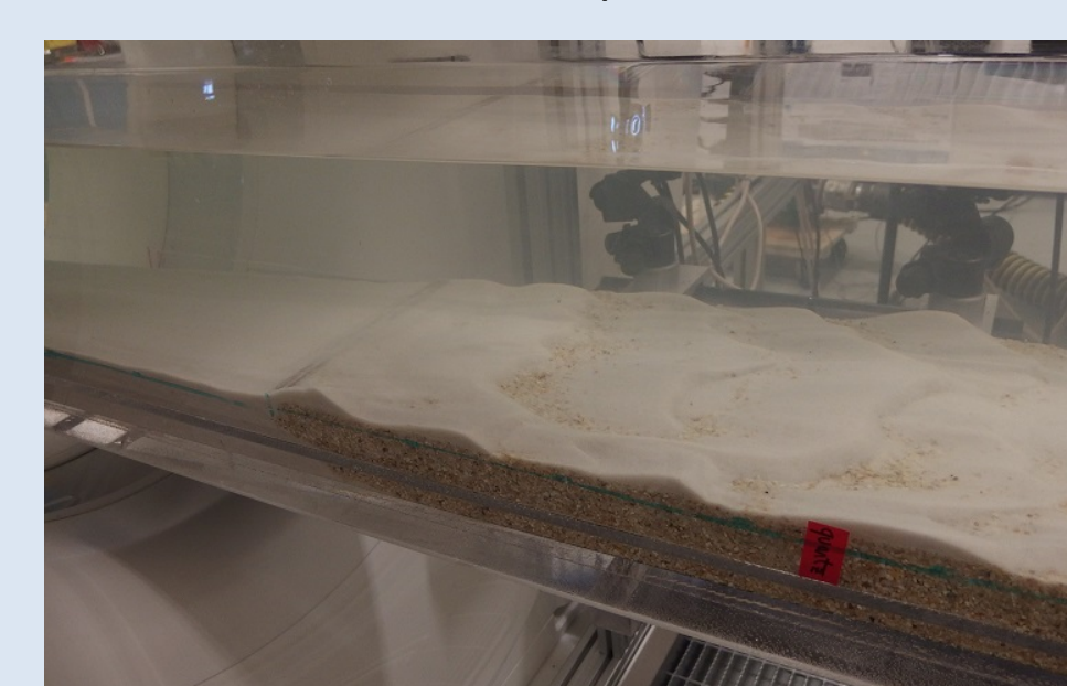
Propagation of fines sands over the coarse sand matrix
