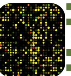
Hybridisation at different temperatures (55, 60, 65 °C) of RNA from biofilms and from reference species : C. reinhardtii, S. vacuolatus Microarray scanning at 5 µm resolution (GenePix 4400A Scanner)
