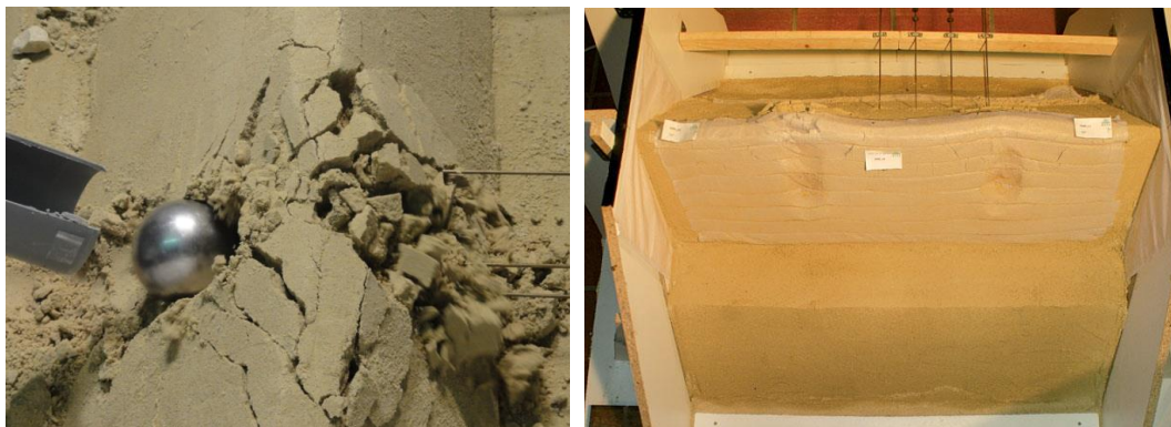
Figure 9 Small-scale experiments conducted by Hofmann and Molk (2013). Left: impact on an unreinforced structure. Right: reinforced structure after two impacts.
