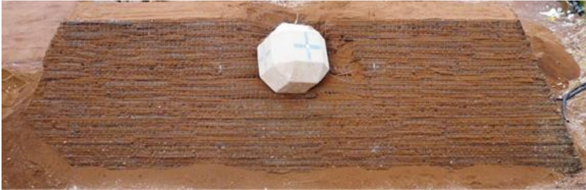
Figure 19 6600 kJ impact experiment conducted by Mongiovi et al. (2013)
