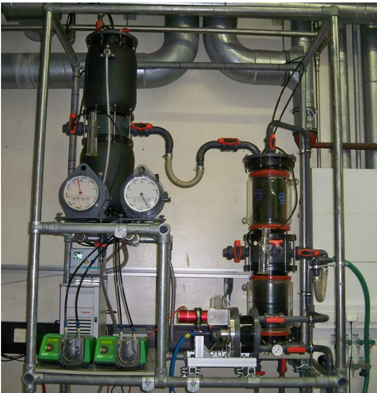
Figure 4: Fermentation plant (pilot scale, 2 x 30-l-reactors)
