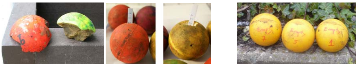
FIGURE 4 Compo-balls after turning (foamy polyurethane on the left and rigid on the right).
