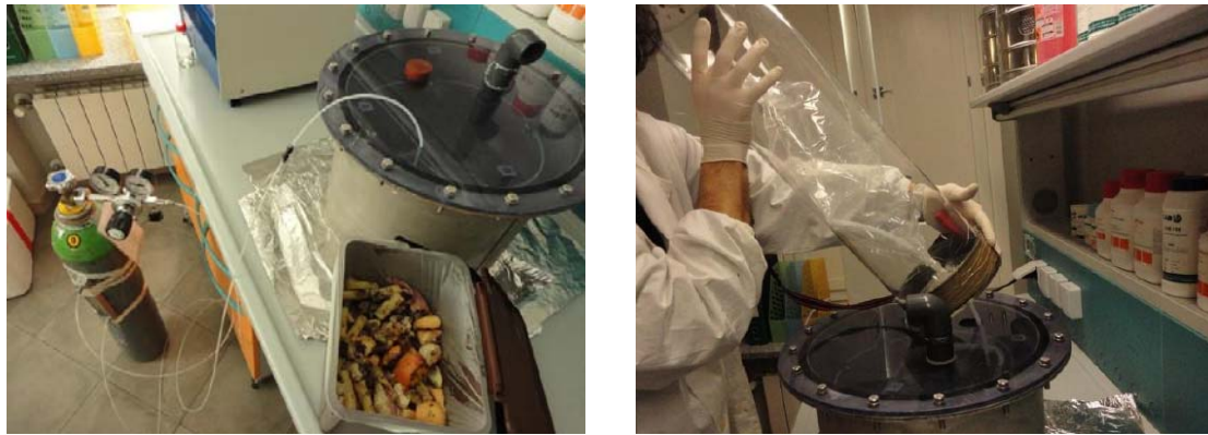
FIGURE 10 Air sampling with a surface emission isolation flux chamber and Nalophan® bags. (M. Giavini et al., 2011).
