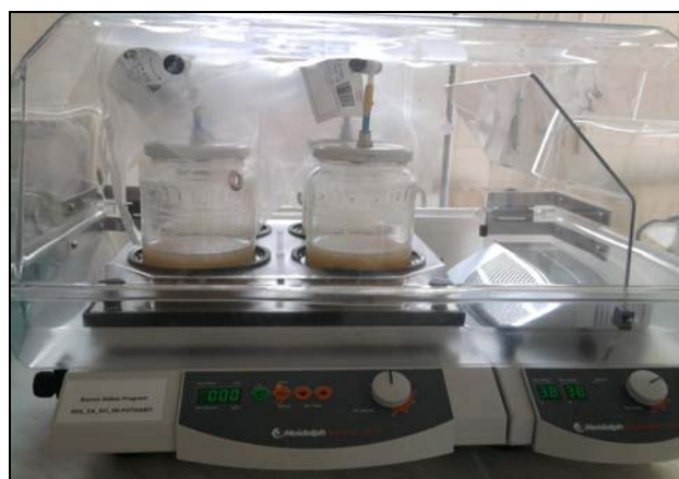
FIGURE 1 Anaerobic hydrolyses model experiment
