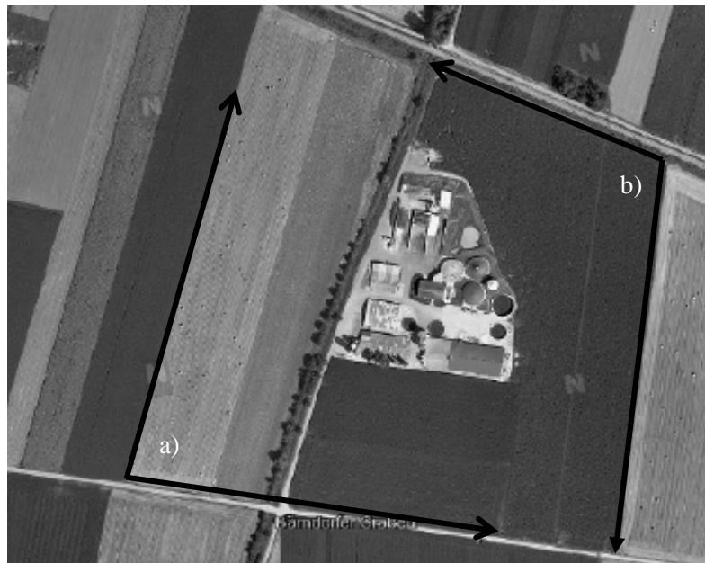
FIGURE 3 Location of the laser lines used for measuring the totality of emissions from the biogas plant depending on the prevailing wind directions (a: NE and E-winds, b: SW and W-winds)
