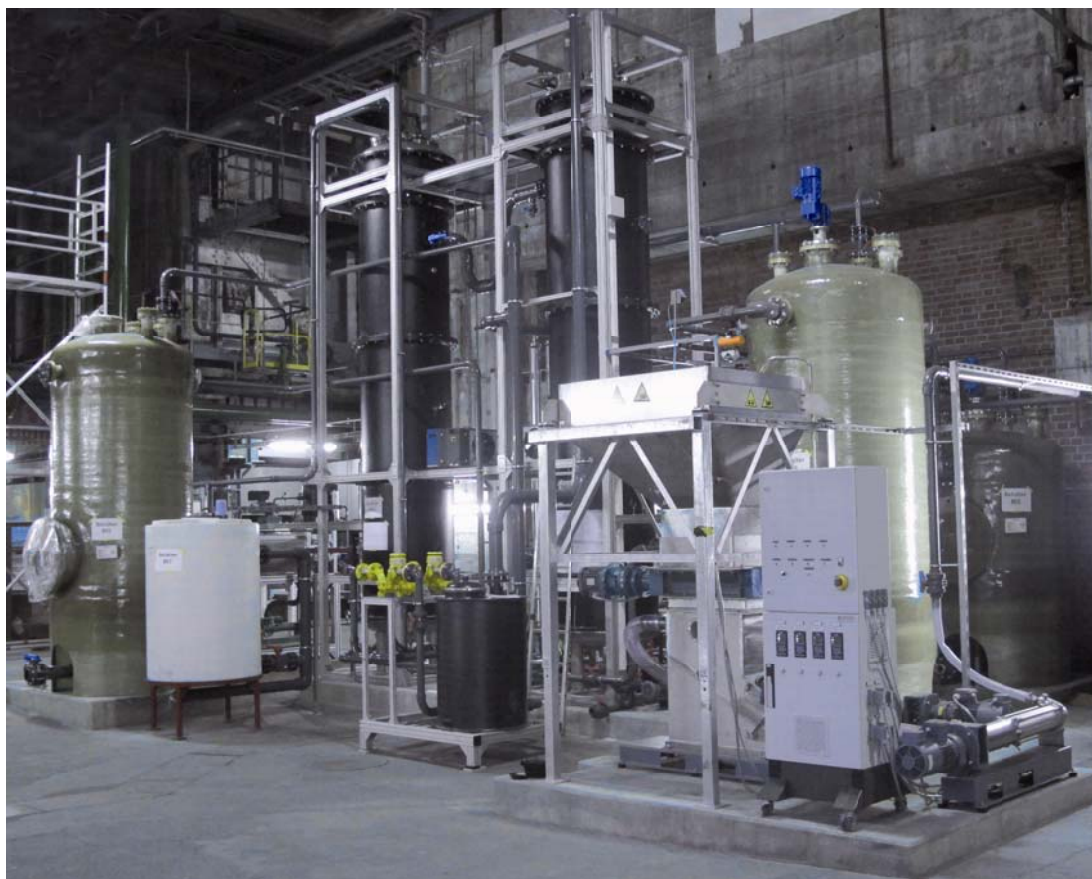
Figure 5: Fermentation plant (demonstration scale, 2x3-5m 3 -reactors)
