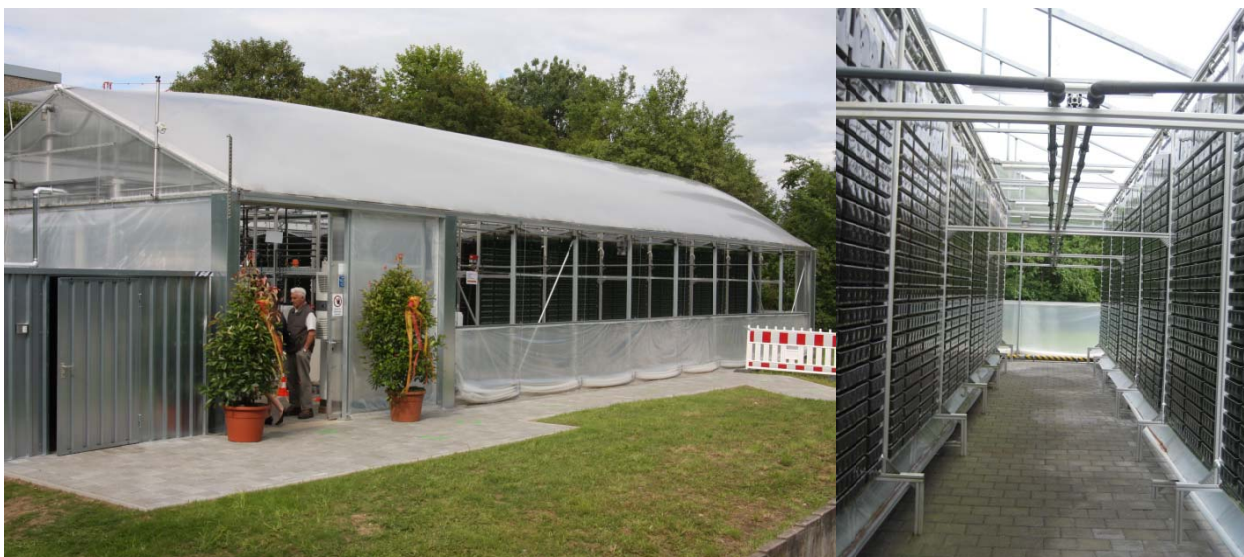
Figure 6: Greenhouse with flat panel airlift photobioreactors
