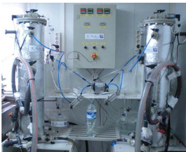
FIGURE 1 Description of the experimental set-up used for the co-digestion studies
