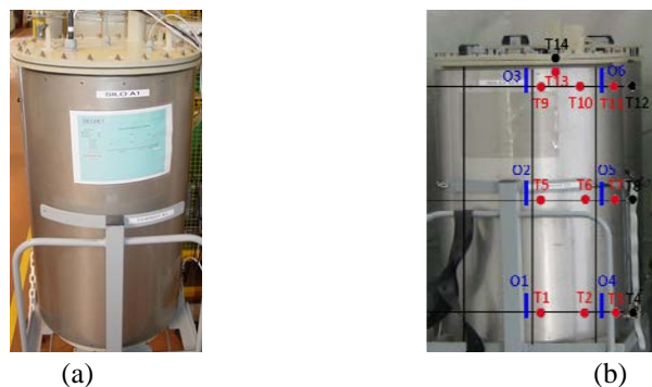
FIGURE 1 (a) Photography of a cylindrical pilot used for the experiments and (b) location of the captors and the probes in the pilot.
