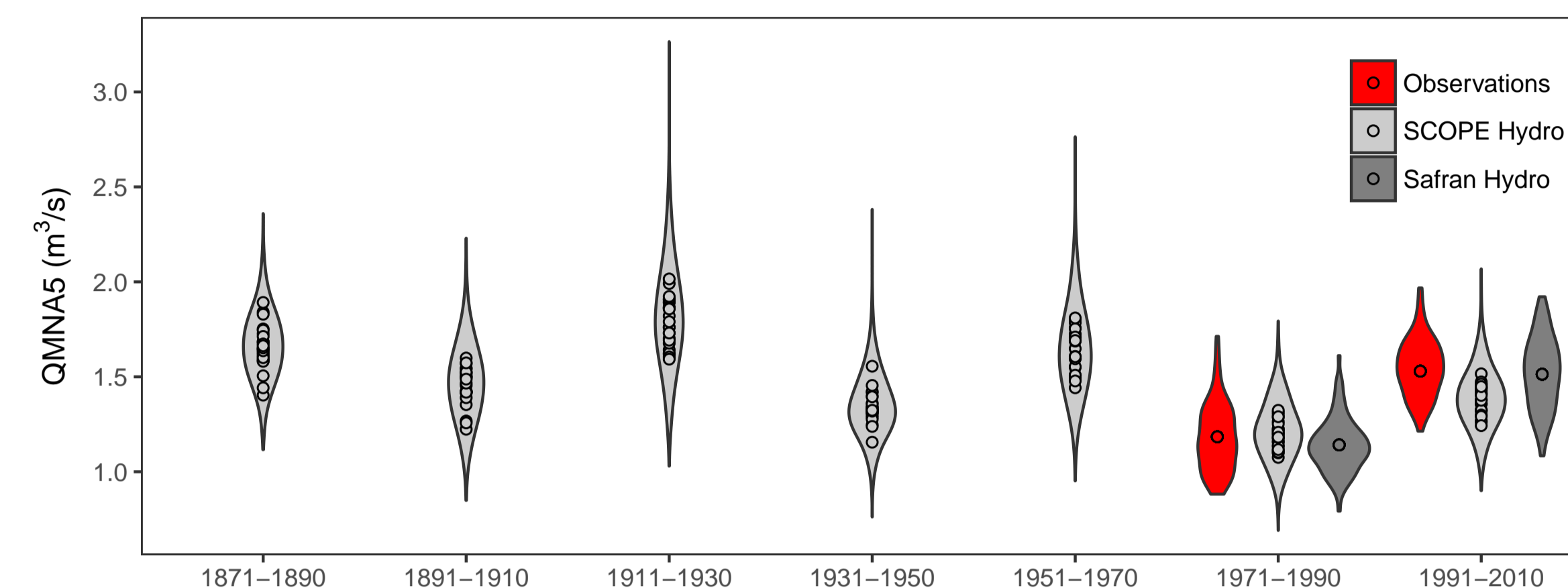
Figure 3: Low-flow values estimated for the Gartempes@Folles catchment, for the 7 time periods and the 3 datasets. Filled points show best estimates for individual series, and violins show the sampling uncertainty (plus downscaling uncertainty for SCOPE Hydro)
