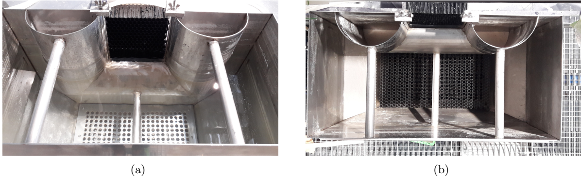
FIGURE 4.2. Tank at the inlet of the street, (a) Initial configuration, with protection grille, (b) Configuration with the plastic grid over the grille.
