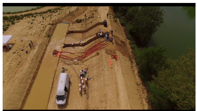
Figure 2. Overview of the site and overflow simulator. The Vidourle River is on the right.
