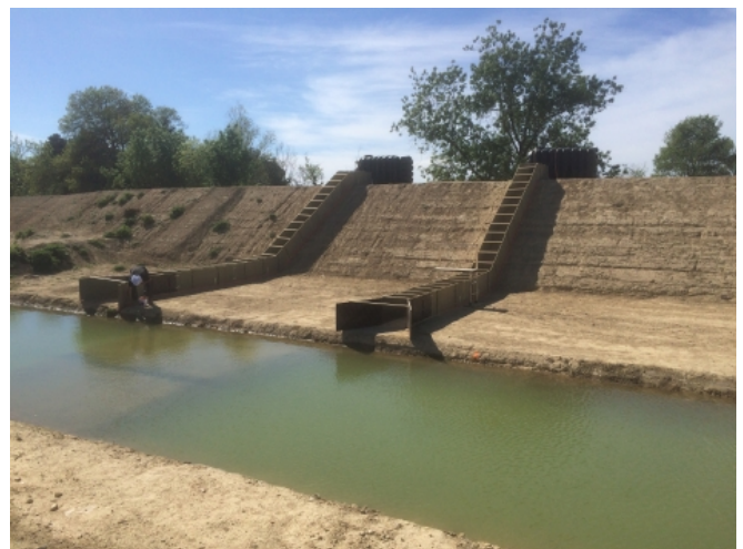
Figure 1. The DigueElite demonstrator, with the two channels before tests, untreated soil on the left, soil-lime on the right.
