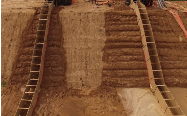
Figure 9. View after the tests campaign. Leaks caused soil erosion on both sides of the canals. Untreated soil being more erodible, erosion on both sides of the canal is more localized and deeper (left). On the contrary, the lime-soil is less erodible, and the leakage flows spread more widely on both sides of the channel (right). On both soils, the erosion of the surface layer highlights the layers of compaction.
