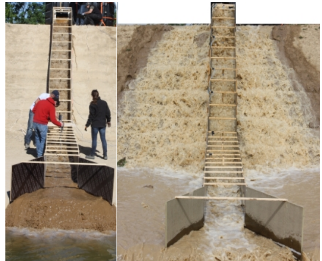
Figure 4. View during test for a flow rate of 95 l/s/mL (minimum flow rate, test No. 1) (left) and a flow rate of 570 l/s/mL (maximum flow rate) (right).
