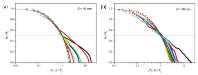
FIG. 11. Semi-logarithmic plot of  $h_f/H_0$  versus  $(T_0-t)/T_2$  for (a) D=10 mm and (b) D=40 mm for the same data and same symbol convention as presented in Fig. 8. The solid line stands for the terminal expansion law given in Eq2 while the dashed line indicates the delimitation  $h_f/H_0=1/2$  used to define  $T_1$  and  $T_2$ .
