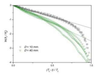
FIG. 9. Plot of natural log of the dimensionless height of the cavity  $h_f/H_0$  vs the dimensionless time  $(T_0 - t)/T_0$  in the regular regime. Data from Fig. 8(a) with D = 10 mm (black open circles) and Fig. 8(b) with D = 40 mm (green open down triangles) restricted to Q > 60 cm<sup>3</sup> s<sup>-1</sup>. The solid lines stand for approximate linear relation with slope equal to -1.6 and -2.5 for D = 10 mm and D = 40 mm, respectively.
