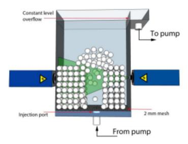
FIG. 1. Schematic of the experimental setup showing the location of the lasers. Flow from the pump is injected at the bottom of the particle bed through a variable diameter injection port. For clarity, only the plane from one laser is depicted in the figure.
