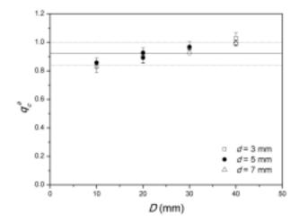
FIG. 19. Adjusted values of the reduced critical flow rate  $q_c^a$  versus D for  $H_0 = 125$  mm and bead diameters d = 3, 5, and 7 mm. The solid line stands for the value expected from the CFD calculation while the dotted lines show approximately the range of variation due to the influence of the injection diameter.
