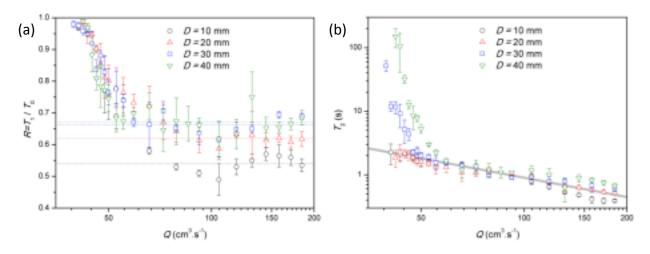
FIG. 10. Semi-logarithmic plot of (a) the ratio  $R = T_1/T_0$  where the horizontal lines stand for the constant value  $R_{\infty}$  reached in the regular regime and (b) the terminal expansion timescale  $T_2$  for d = 3 mm,  $H_0 = 125$  mm and D = 10, 20, 30, and 40 mm. The solid line in grey stands for an empirical expression  $T_2 \propto Q^{-1}$  with a coefficient equal to 90 cm<sup>3</sup>.
