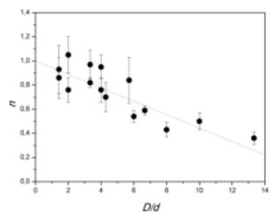
FIG. 16. Plot of the exponent *n* versus the ratio D/d for all the data. The dotted line stands for the linear relation:  $n = 1 - \frac{D}{18d}$ .
