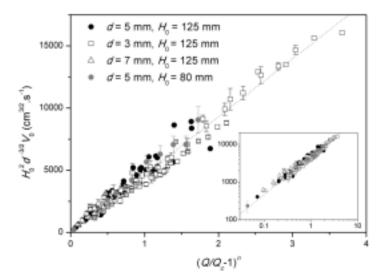
FIG. 15. Plot of  $H_0^2 d^{-3/2} V_0$  versus  $(Q/Q_c - 1)^n$  for all the data. The dotted line stands for a proportionality relation with a coefficient  $B \sim 4650$  cm<sup>3/2</sup> s<sup>-1</sup>. Inset: same data in log-log representation.
