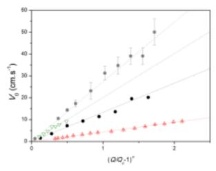
FIG. 13. Typical evolution of the mean expansion rate  $V_0$  versus  $(Q/Q_c-1)^n$  for the same data as in Fig. 12 using the same nomenclature. The values for n are the ones found in the nonlinear regression analysis in Fig. 12.
