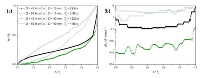
FIG. 6. Plot of (a) the normalized fluidized height  $h_f/H_0$  and (b) the rate of expansion  $dh_f/dt$  versus the normalized time  $t/T_0$  for d=3 mm,  $H_0=125$  mm and D=10 mm (black circles) or D=40 mm (green down triangles). Typical expansions in the regular and the ultra-slow regimes are observed for Q=65.8 cm<sup>3</sup> s<sup>-1</sup> (open circles) and Q=43.4 cm<sup>3</sup> s<sup>-1</sup> (closed triangles), respectively.
