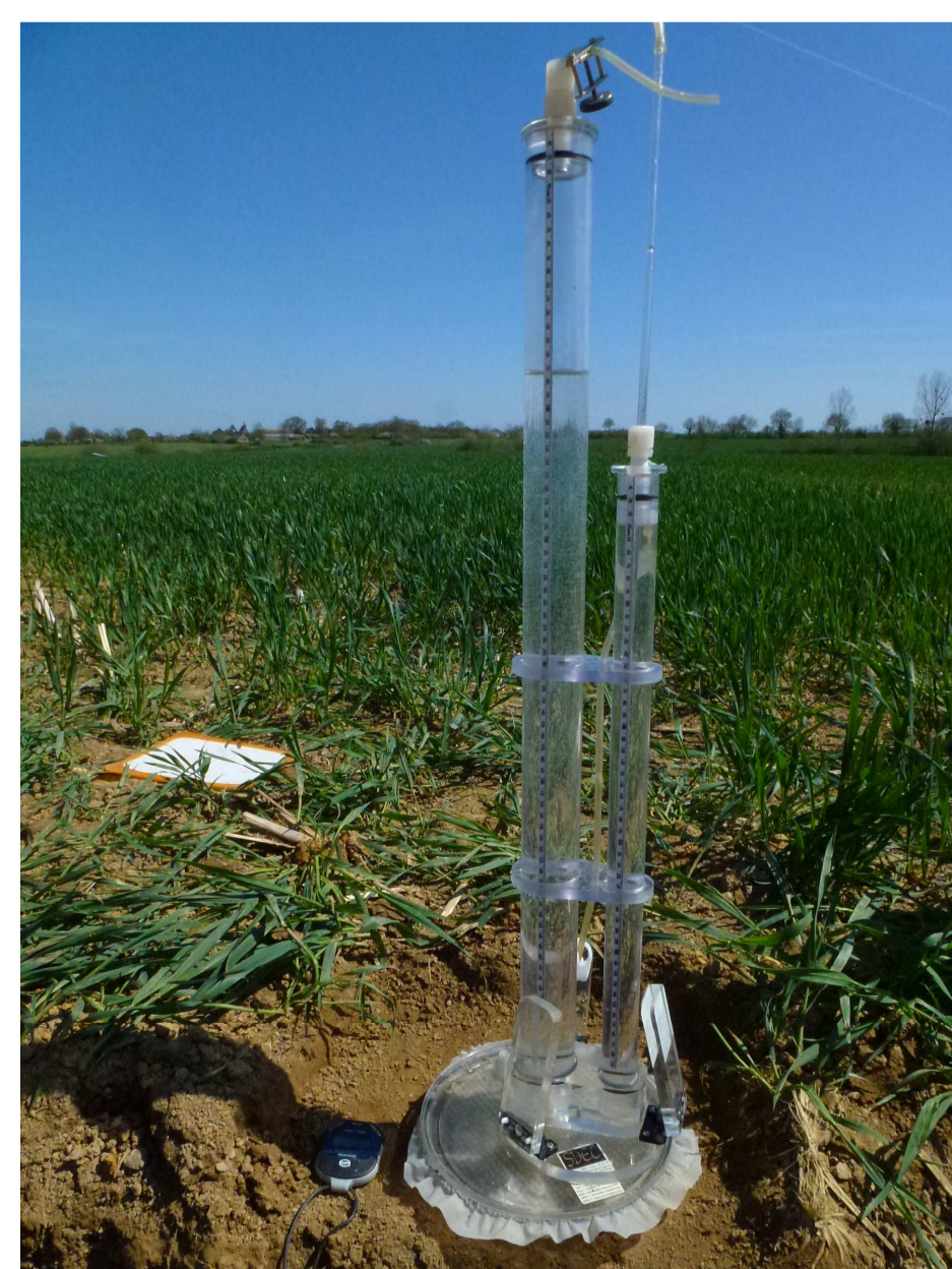
Photo 2 : Tension Disc infiltrometry on the surface plough layer, April 2013.
