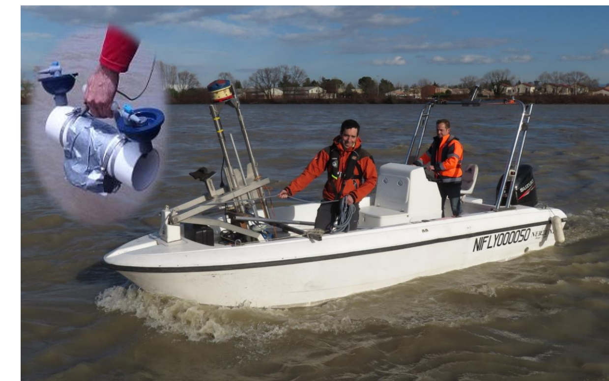
CNR vessel mounted ADCP for mobile deployments and Niskin bottle ready to be used.
