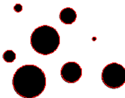
Figure 3. Synthetic particles image and contours (red) determined by shadow processing
