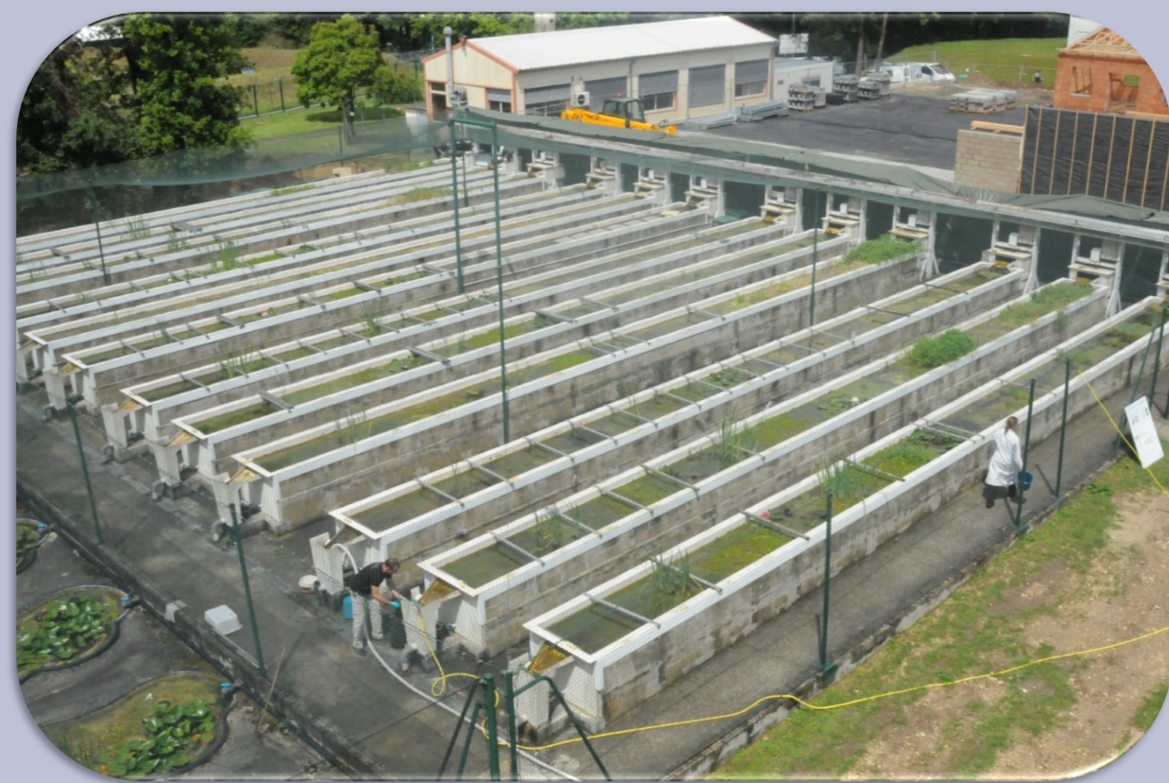
Figure 1 : The mesocosm platform with 12 lotic mesocosms of 20 m long and 1 m wide
