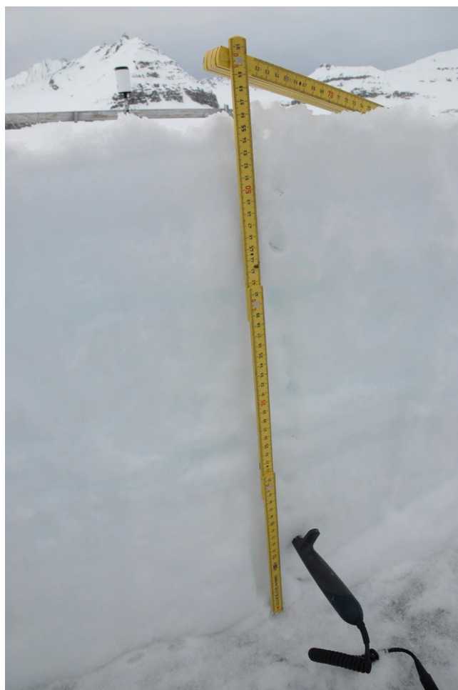
Figure E4. Measuring snow temperature in profile, 10 May 2016. Data can be found in Table E1.
