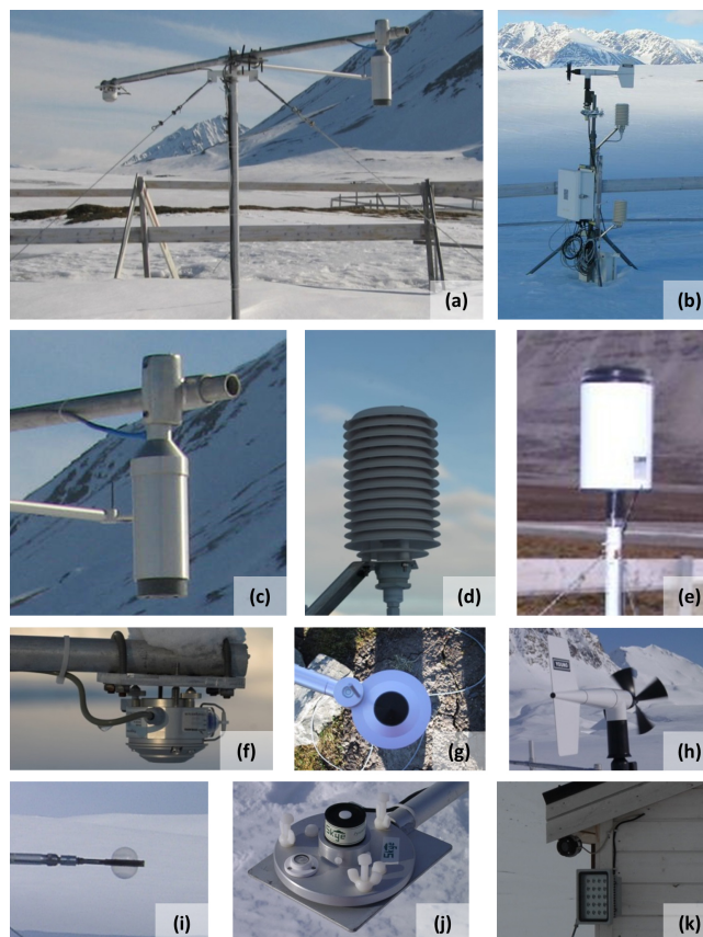
Figure C2. Climate station, Bayelva, September 1998–August 2009. (a) Radiation–snow tower, (b) meteorological tower, (c) snow height sensor (from September 1999: 2 m; from July 2001: 1.6 m; from September 2003: 1.45 m), (d) temperature–relative humidity (2 m) and temperature (1 m) sensor, (e) rain gauge (1.68 m top of bucket above ground level), (f) pyrgometer (from May 2003: 2 m; from September 2003: 2 m) installed in May 2002, (g) net radiometer (from April 2000: 1.14 m; from September 2003: 1.6 m), (h) wind speed and wind direction sensor (3 m), (i) net radiation sensor (from April 2000: 1.14 m, from September 2003: 1.6 m), (j) pyranometer (2 m) and (k) camera (2 m) with flash since August 2013. Sensor details can be found in Table 2.
