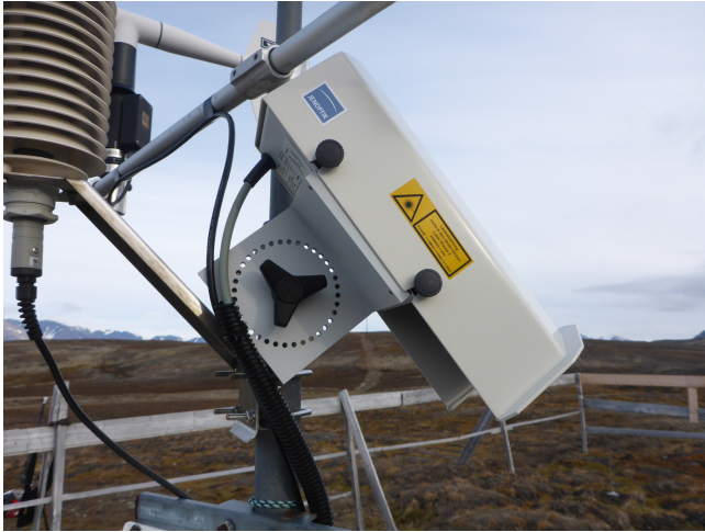
Figure C4. Laser snow depth sensor attached to the climate station, Bayelva, August 2013–present, (78.92094° N, 11.83334° E).
