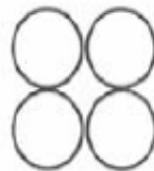
a. cubically packed uniform spheres,  $\phi = 48\%$
