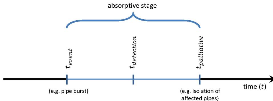
**Figure 3:** Disruptive events in WDS; absorptive stage - times.
