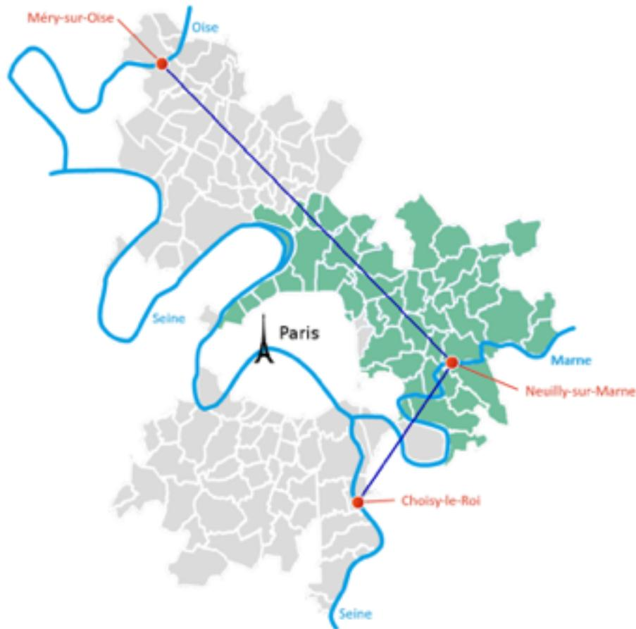
**Figure 7:** The SEDIF perimeter around Paris, the three main drinking water treatment plants in red and their interconnections in dark blue.
