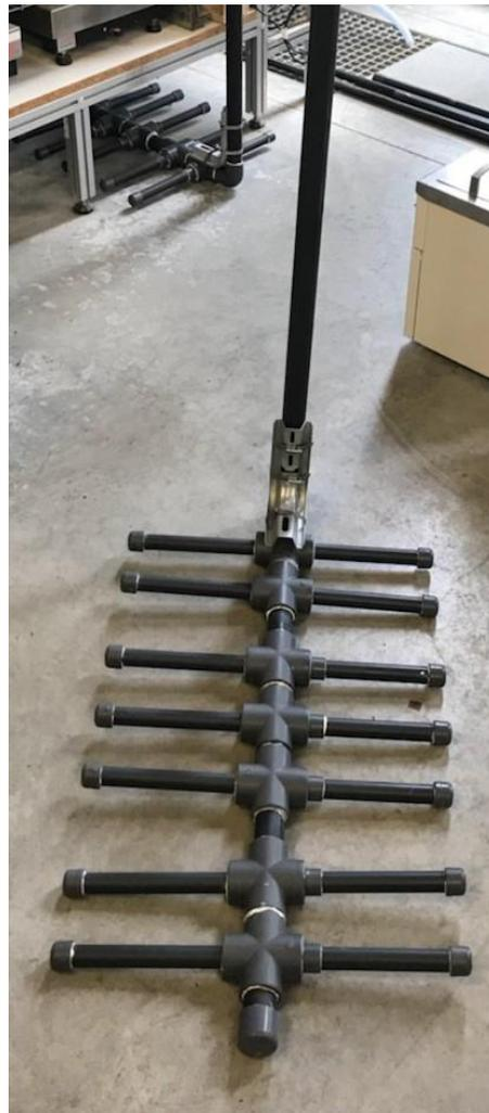
**Figure 14 Diffuser used in the reactor'**
