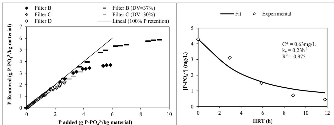
**Figure 3. Left: Evolution of P retention efficiency of filters B, C and D (\*DV: Dead volume); Right: Model fitting for filter C at an estimated saturation level of 2,7gP/kg material considering DV (Campaign of Octobre 2017)**
