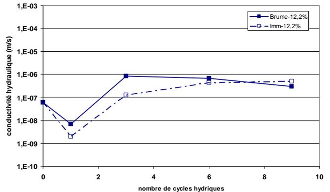
FIGURE 8 : CONDUCTIVITE HYDRAULIQUE A 10 °C OBTENUE PAR ESSAI DE PERMEABILITE A CHARGE CONSTANTE SUR DES EPROUVETTES DE SOL COMPACTE A  $w = 12,2 \%$ , AYANT SUBI UN PROCESSUS DE DEGRADATION PAR IMPOSITION DE CYCLES DE SECHAGE ET HUMIDIFICATION EN ATMOSPHERE HUMIDE (BRUME) OU REMONTEE CAPILLAIRE (IMM)
