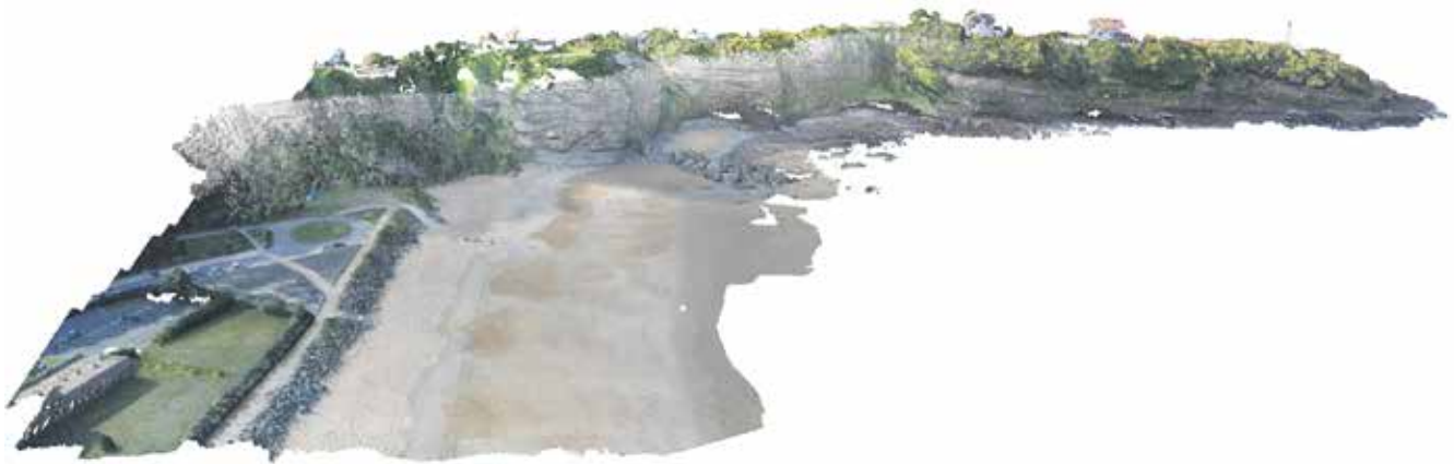
Figure 4. Numerical model of terrain obtained by drone image photogrammetry of the beach and cliff at Cap Saint-Martin (Anglet and Biarritz, Pyrénées-Atlantiques; achieved by V. Marieu)
