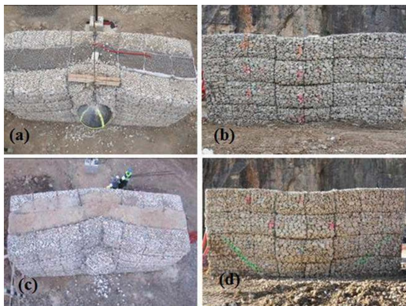
Fig. 6. Views of (a, c) the uphill face and crest and (d, b) the downhill face of structures (a, b) BA and (c, d) STM after the 2000 kJ kinetic energy impact test. [Colour online.]
