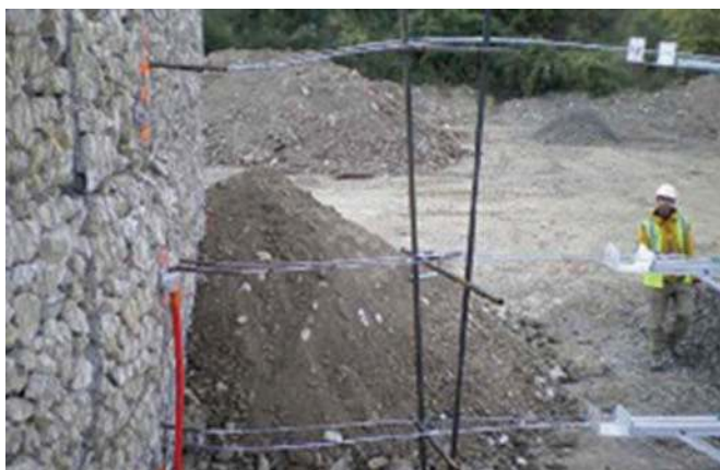
Fig. 4. Deformation of displacement sensor extension rods after the third impact on structure BA (i.e., ballast). [Colour online.]
