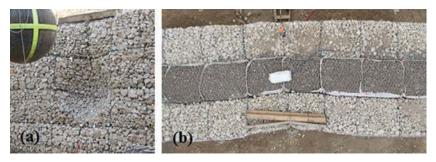
**Fig. 6.** Views of (*a*, *c*) the uphill face and crest and (*d*, *b*) the downhill face of structures (*a*, *b*) BA and (*c*, *d*) STM after the 2000 kJ kinetic energy impact test. [Colour online.]
