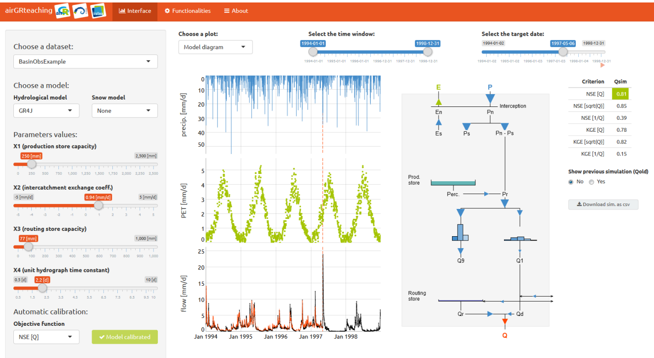
Figure 6. The airGRteaching interface that is used for teaching hydrological modelling. Students can choose a catchment dataset and a hydrological model and activate a snow model on the top left panel of the interface. Modifying the parameters values (on the left) by using the sliding bars will automatically update the graphs and scores displayed (on the right). This interface highlights in an interactive manner the basic principle of the rainfall–runoff relationship and its description in hydrological models. At the bottom left of the interface, an objective function can be chosen and an automatic calibration procedure can be launched within the interface.
