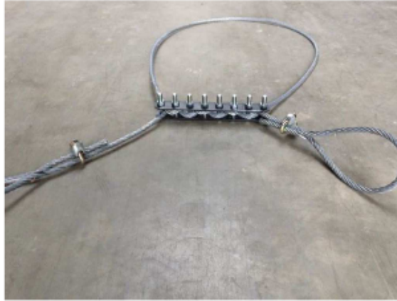
Figure 3: Friction energy dissipating device (GTS).
