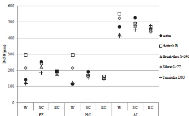
FIGURE 4 : EFFET DES ADJUVANTS, DU TYPE DE BUSE ET DE LA FORMULATION DE PHENMEDIPHAM SUR LA TAILLE DES GOUTTES. ACTIROB (METHYLESTER DE COLZA), BREAKTHRU (POLYETHER TRISILOXANE), SILWET L77 (HEPTAMETHYLTRISILOXANE), TENSIOFIX D03 (NON IONIQUE) (FF : JET PLAT, HC : CONE CREUX, AI : INDUCTION D'AIR), (W : EAU PURE, SC : SUSPENSION CONCENTREE, EC : EMULSION CONCENTREE) (ALHEIDARY *ET AL.*, 2016, D'APRES STAINIER *ET AL.*, 2006).
