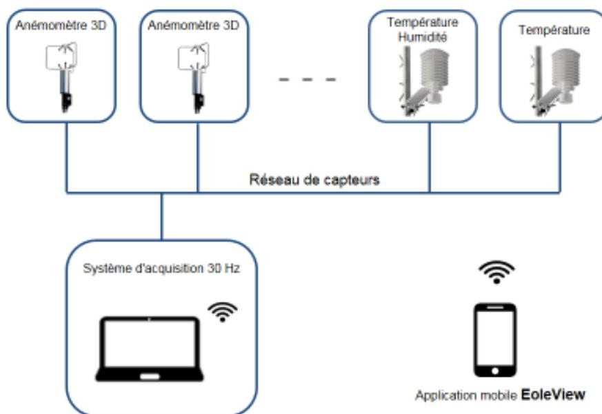
**FIGURE 14 :** REPRESENTATION SCHEMATIQUE DE RESEAU DE CAPTEURS METEOROLOGIQUES IMPLANTES SUR LA PLATEFORME DU BANC D'ESSAI EOLEDRIFT, POUR LE CONTROLE DE LA CONFORMITE DES CONDITIONS DE MESURE ET LA TRAÇABILITE DES ESSAIS.
