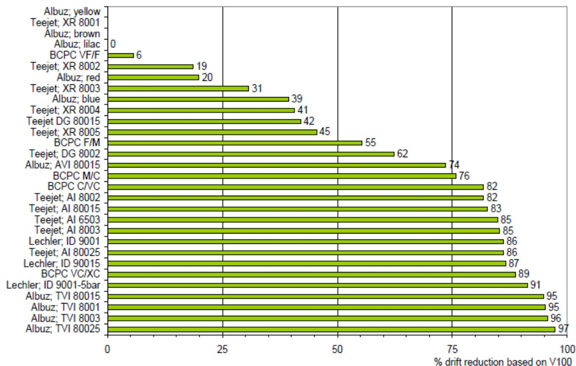
**FIGURE 6 : TAUX DE REDUCTION DE DERIVE POTENTIELLE BASE SUR LE V100 (% DU VOLUME DE BOUILLIE PULVERISEE DONT LES PARTICULES ONT UN DIAMETRE < 100  $\mu$ M) RELATIVEMENT A LA REFERENCE ALBUZ YELLOW AVEC DE L'EAU (VAN DE ZANDE *ET AL.*, 2008).**
