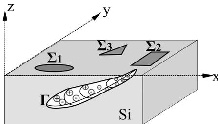
Figure 1. Schematic representation of a volume ( $\Gamma$ ) of apparition of electron-hole pair (white in the drawing) in a silicon substrate (light grey). The three collecting surfaces represented here ( $\Sigma_1$ ,  $\Sigma_2$ ,  $\Sigma_3$ ) are arbitrarily shaped and as numerous as wanted
