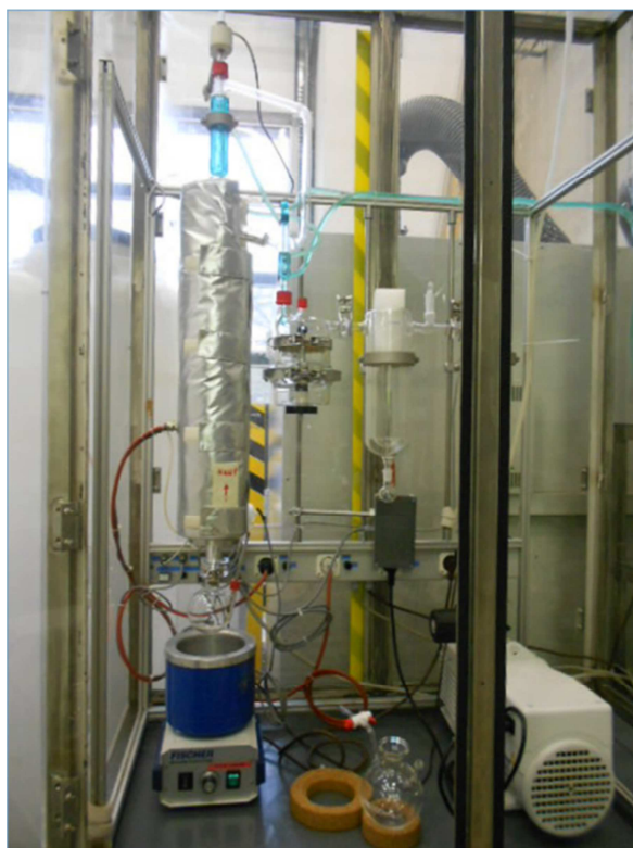
Fig. 7. Experimental batch distillation column. Model LABODEST® HRS 500C of Fischer Technology.
