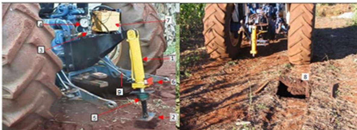
Figure 1. Soil compaction test in-situ with plate penetrometer: 1 hydraulic cylinder, 2 plate, 3 pressure control valve, 4 manometer, 5 load cell, 6 displacement sensor, 7 datalogger, 8 sinkage, 9 device for adjusting the vertical position of the plate with the horizontal plane of the ground.
