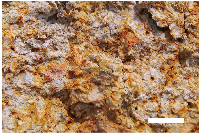
Figure 3. Close-up photograph of the typical soil structure in the subsoil horizons of the Ban Nabone site showing oxidized micro-domains (mostly along cracks and around root channels) in brown-red colours immediately adjacent to reduced micro-domains where greyish colours prevail. The white horizontal bar to the bottom right of the photograph represents 5 mm.
