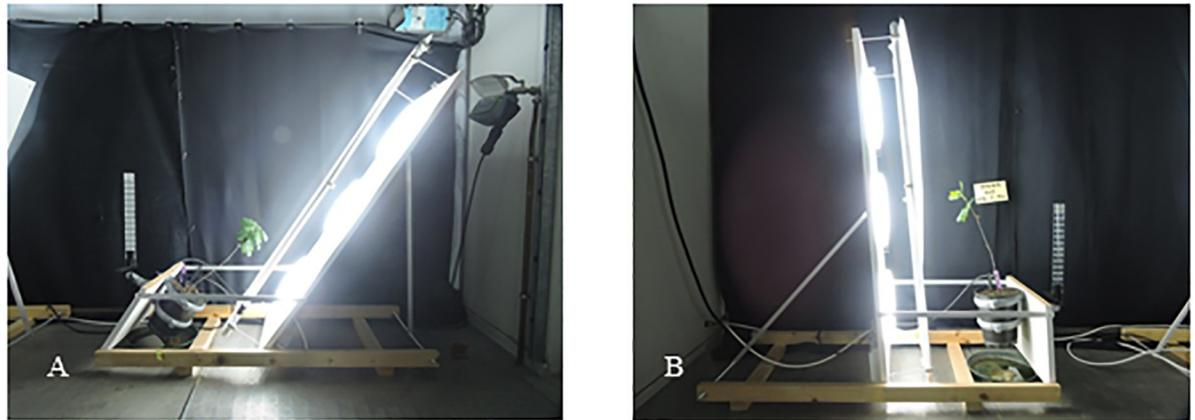
**Fig 3. Side views of the anisotropic light device installed in a growth chamber.** A: Young oak is installed on the anisotropic light device tilted 35° from the vertical. B: Young oak is installed on the anisotropic light device tilted 5° from the vertical. The walls of the growth chamber were covered with black curtains in order to avoid light reflection.
