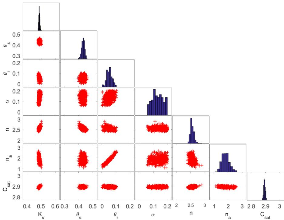
**Figure 5.** MCMC solutions in which calibration is performed using only SP data located 5 cm from the surface. The diagonal plots represent the posterior probability distribution of the parameters. The off-diagonal scatterplots represent the pairwise correlations in the MCMC drawing.
