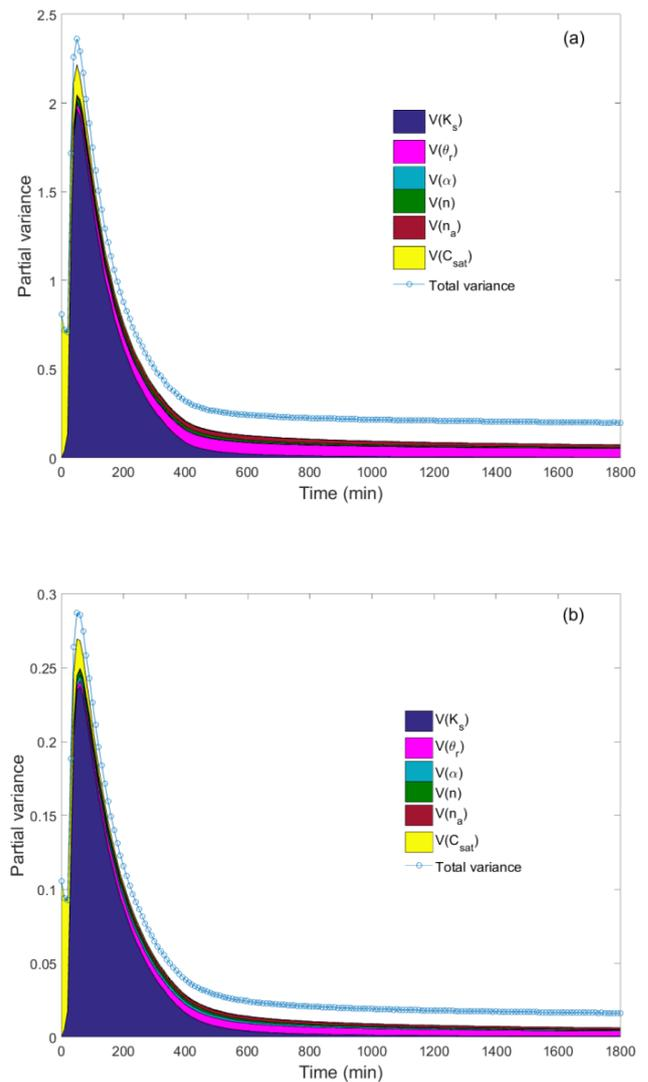
**Figure 3.** Time distribution of the SP variance at 5 cm (a) and 77 cm (b) depth. The shaded area under the variance curve represents the partial marginal contributions of the random input parameters; the contribution of interactions between parameters is represented by the blank region between the shaded area and the variance curve.
