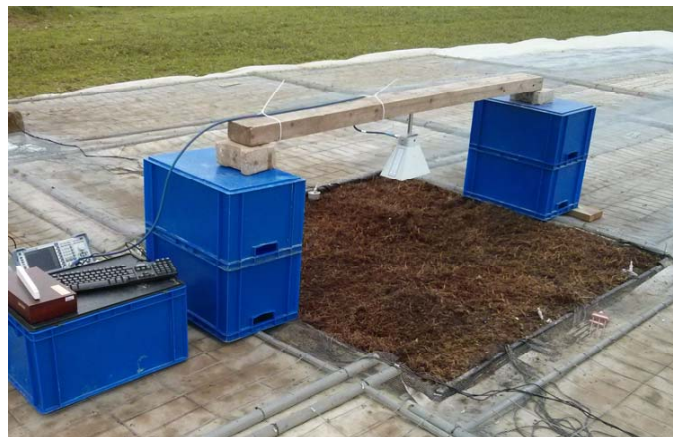
Figure 5. Pictures of the off-ground ground-penetrating radar (GPR) system fixed above the organic soils (with the vegetation layer removed) consisting of a vector network analyser connected to a horn antenna with a low-loss N-type 50 \Omega impedance coaxial cable.
