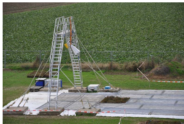
Figure 3. The Selhausen remote sensing field laboratory (Germany) consisting of an L-band radiometer (yellow box + conical horn antenna) fixed at 4 m height on an aluminium arc and a sand box covered by the soil–vegetation blocks in the centre of a wire grid.
