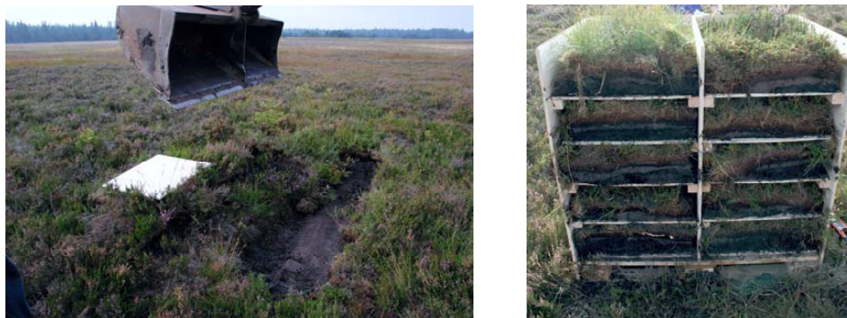
Figure 2. Undisturbed soil–vegetation blocks excavated using a hydraulic excavator from the HOBE heathland test site in the Skjern River catchment, Denmark (left), and transported in wooden boxes (right) to the Selhausen remote sensing field laboratory in Germany .
