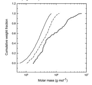
Fig. 3. Cumulative molar mass distributions obtained by AF4-MALLS of 0.5% (w/w)  $\kappa$ -carrageenan solutions without SSL (continuous line), with 0.004 and 0.017% SSL (dashed and dotted line, respectively).
