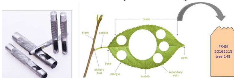
Fig. 3. Calibrated leather puncher (left) and leaf punched for LMA determination. Two punches are used in this example, with area a_1 (small) and a_2 (large), respectively.
