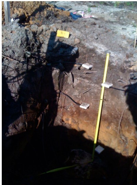
Figure 3. Installation of the soil moisture sensors at Hermitage site.
