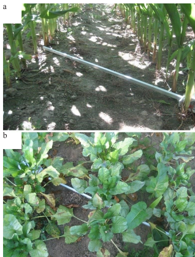
Fig. 4. Example of a below-canopy probe position in: a – a maize crop and b – a beet crop.
