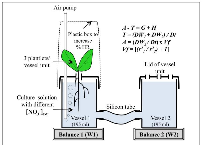
FIGURE 2 | The principle of gravimetric device to measure simultaneously water uptake (A), transpiration (T) and shoot growth (G) and capacitance (H). Vf is a vessel factor depending on the radius of vessel 1 (r1) and vessel 2 (r2). Note that the bubbler constantly renews the air in the closed plastic chamber and creates a slight overpressure.
