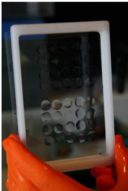
Fig. S1. Gelbond® film with 40 gels, attached to a plastic frame with metal hooks in each corner.
