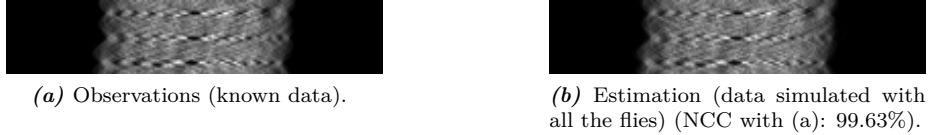
Figure 20: Sinograms from Figure 21a corresponding to the hot rod phantom with a low resolution and with noise. Images with 185 pixels per projection, 1 st angle: 0°, angular step: 5°, and last angle: 175°.
