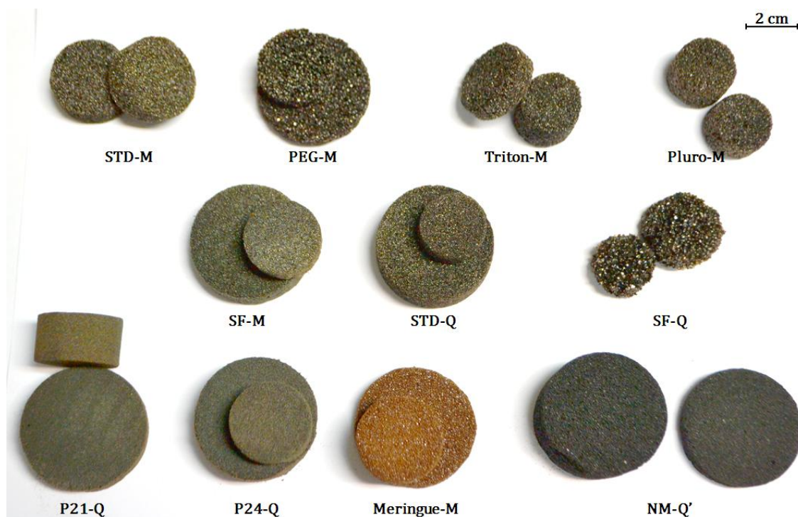
Fig. 1. General view of all tannin-based foam samples studied in this work.
