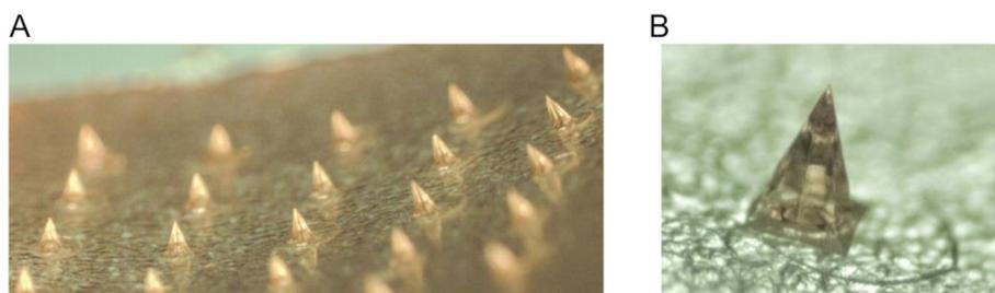
**Fig. 1.** DNA-loaded dissolvable microneedle patches. (A). An image of the array of needles. Each patch was 9 cm<sup>2</sup> and comprised of 225 microneedles. (B). An image of a single microneedle that is 500 μm in height and has a base of 333 μm diameter. DNA was loaded throughout the entire microneedle.
