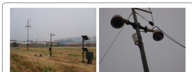
Fig. 4 Imaging device in the Zhengzhou, Henan Province. The main components include a high resolution CCD digital camera (E450 Olympus) and low-resolution monitoring equipment. The camera is set 5 m high above the ground
