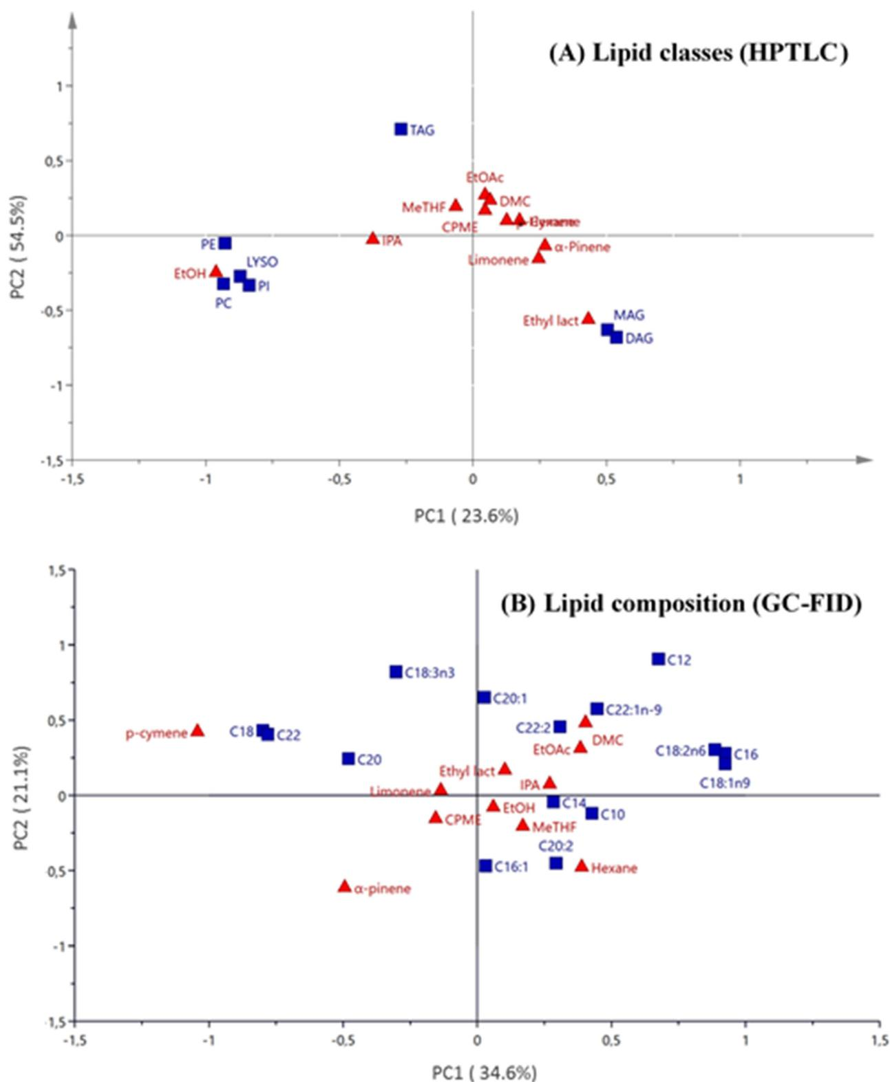
**Fig. 1.** Principal component analysis biplot (score and loading values) represented by PC1 versus PC2 for (A) lipid classes obtained by HPTLC and (B) lipid composition obtained by GC-FID, and tested solvents.
