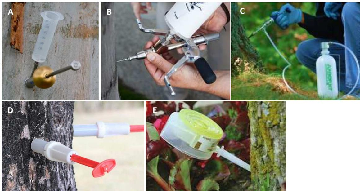
217 Figure 1: Existing trunk-injection devices. (A) Bite®, (B) Wedgle® Direct-Inject System, (C)
