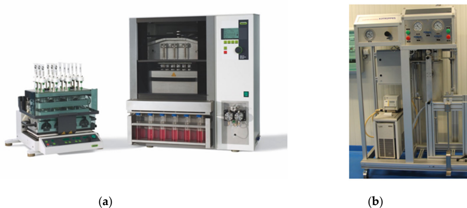
Figure 2. Subcritical water extraction system. (a) laboratory scale ( www.buchi.com ). (b) pilot scale ( www.zippertex.com ).
