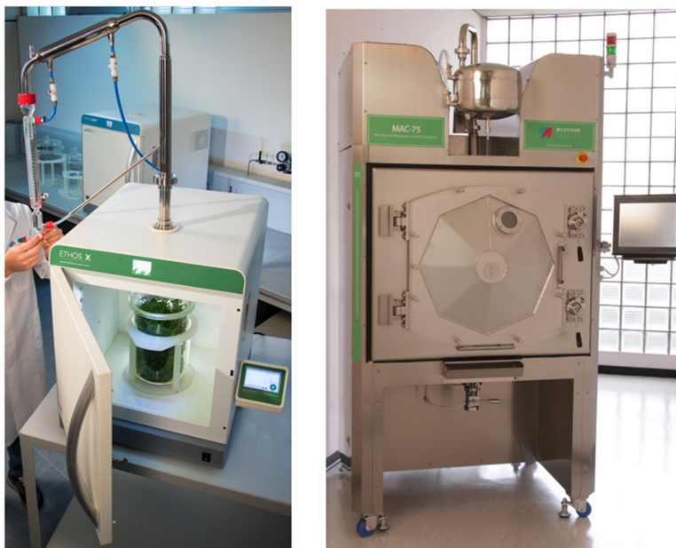
Figure 1. Microwave solvent-free extraction: From analytical lab to industrial scale.
