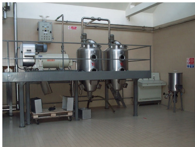
Figure 6. Industrial scale ultrasound extraction process (2 × 500 L) as intensification technique for extraction using vegetable oils (Reus— www.etsreus.com ).
